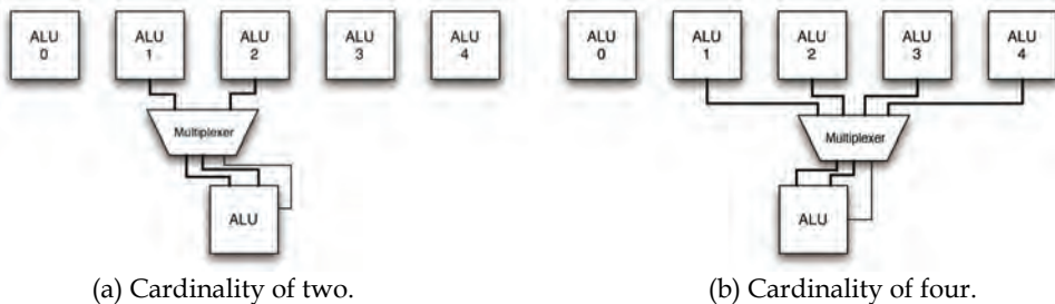
Fig. 4. Interconnects of two different multiplexer cardinalities.
