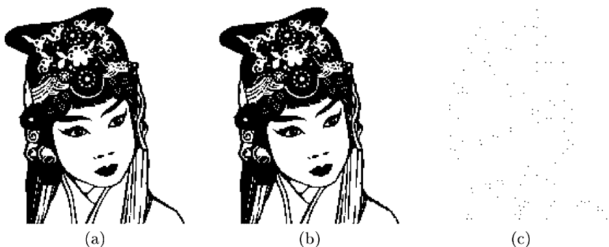
Fig. 4. Data hiding by our method. (a) the original host image with size 166 \times 198 , (b) the marked image after embedding 200 bits, (c) the difference map, indicated by black pixel (totally 105 pixels).
